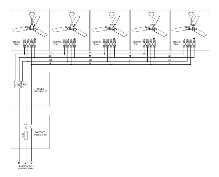
THE CONTROLLER IS FITTED WITH AN INTERNAL FUSE TO PROTECT CONTROLLER WIRING AND COMPONENTS. IT IS NOT DESIGNED TO PROVIDE MOTOR OVERLOAD PROTECTION, ADDITIONAL CONTROL EQUIPMENT IS NECESSARY FOR THIS FUNCTION.
